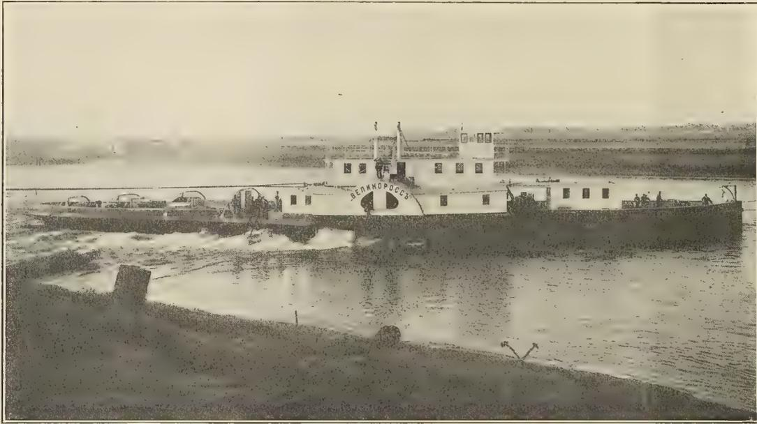
WELIKOROSS, AN 800-HORSEPOWER DIESEL-ENGINED RIVER TUG. MANY VESSELS OF THIS TYPE ARE IN SERVICE ON THE VOLGA
